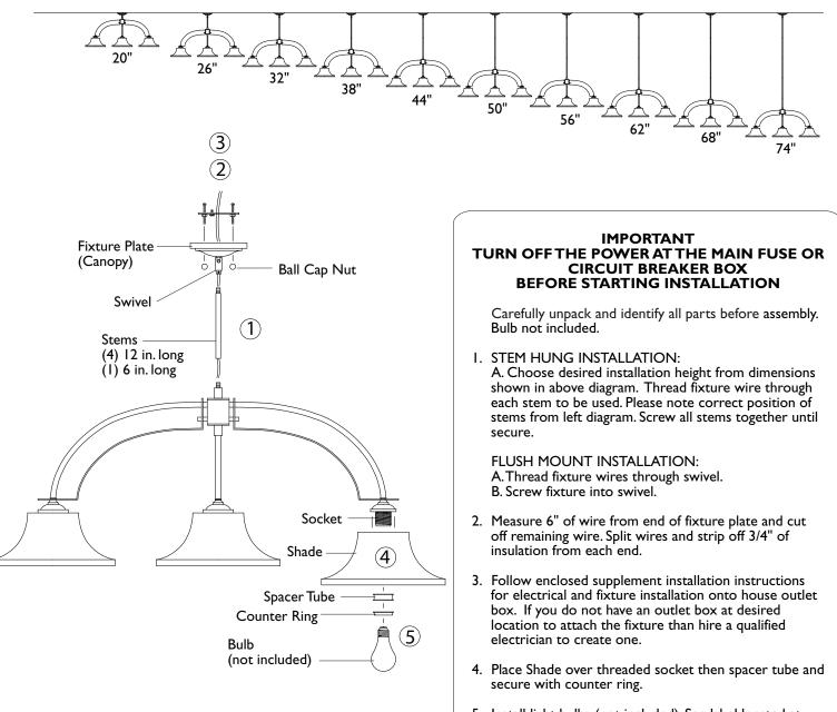
5. Install light bulbs (not included). See label located at socket area for type and maximum allowed wattage.
