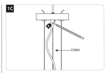
NOTE:The power cord does not support the fixture. For a casual "lazy cord" look, cut the power cord several inches longer that the drop height of the fixture.
