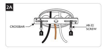
1 Mount the crossbar to the electrical box with the two provided #8-32 screws.
