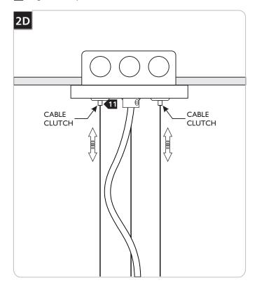
11) Adjust the aircraft cables until the fixture is level; feed the cable into the cable clutch to raise the fixture and push in on the cable clutch nipple to release the cable and lower the fixture.
