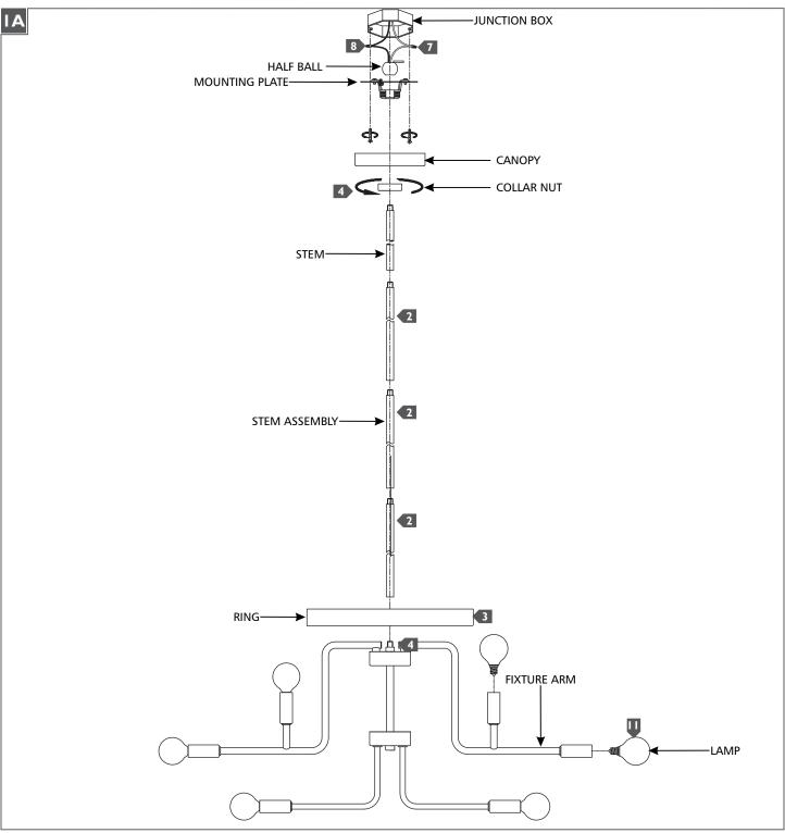
Screw the half ball to the stem which will be on top.
