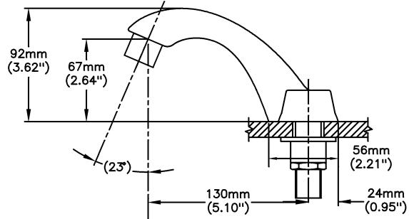
INLETS: 1/2" MIP/COUPLING NUTS (NUTS NOT SUPPLIED)
