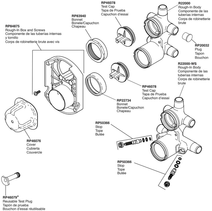
\*Used to plug one inlet side (Hot or Cold) to prevent cross flow when checking for leaks before the cartridge is installed. Insert into the inlet, place test cap and use the bonnet to secure in place.
