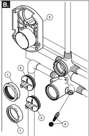
**A.** Connect valve body to water supplies using the proper fittings for your valve body type (copper tubing, iron pipe or Pex).
