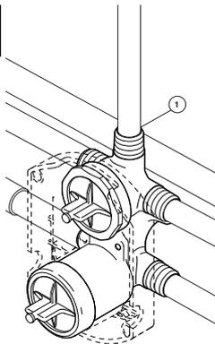
Connect top outlet port (1) to shower pipe with proper fittings.
