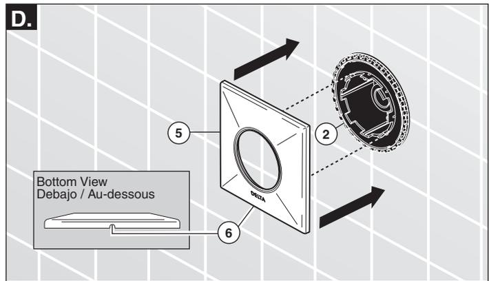
**C.** Apply the provided 100% plumbing silicone / adhesive (4) to the indicated flat surface of escutcheon (5) as shown. Take care not to cover the weep hole (6) with silicone/adhesive by leaving a 1/4" gap on either side of the hole.
