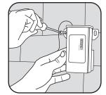
Insert anchors into holes and mount LTPS unit to wall with supplied screws.
