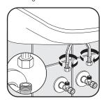
7. Connect braided hose with filter to supply valve. Cold water line has a white label.
