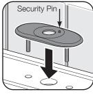
1. Mount cover plate if required. Use silicone caulk to seal plate to the sink. Security pin should be on the right side.
