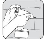
1. Position LTPS unit on wall and mark mounting holes on mounting surface.
