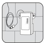
Connect spout wire to LTPS connector wire, making sure connectors are oriented correctly.
