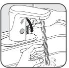
2. For faucets with external mixer installed, turn mixer handle from cold to warm. You should feel the water temperature increase.
