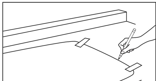
Draw a line parallel to the front edge of the countertop, indicating how far back the sink should be located. Typically the setback is 2" to 2-1/2" from the front of the counter, depending on the countertop overhang, the type of sink bowl and the size of the sink deck.
