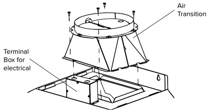
2. Fit the vent system over the exhaust outlet.
