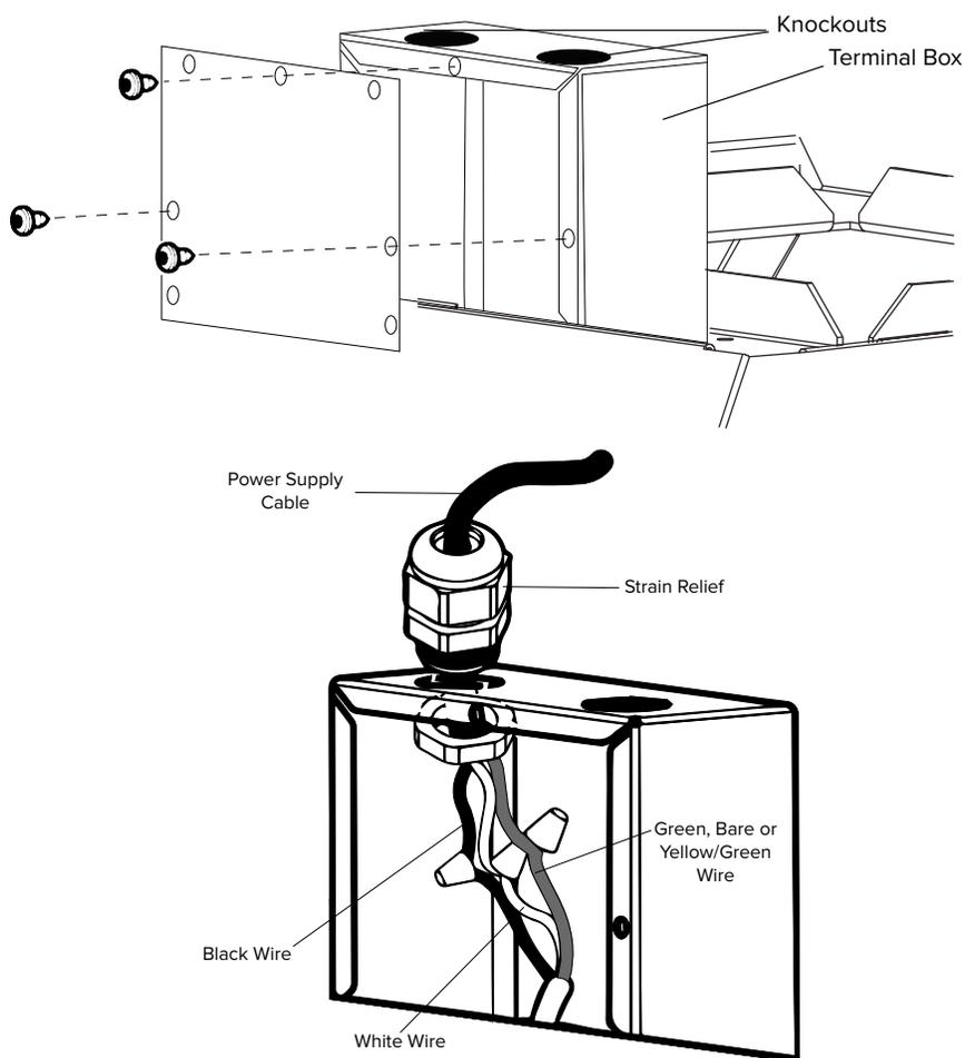
5. Use a UL listed wire connector and connect the black wires together.
