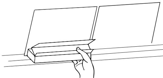
4. Wash the metal filters and grease trays in the dishwasher at low heat or soak in hot, soapy water.
