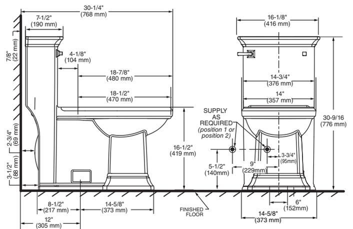
**IMPORTANT:** Water supply on the wall is required at 3-3/4" or 9" from centerline of the toilet (see rough-in). First suggested position is hidden behind the toilet. The geometry of the toilet gives space for this installation. The second suggested position is next to the toilet. Between these two positions, the space for the supply between wall and toilet is limited to 3-1/4". In this case, check your supply and hose dimensions.
