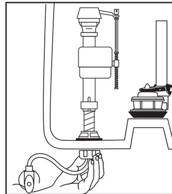
With correct washers in place (see Step 8a), tighten COUPLING NUT 1/4 turn beyond hand tight.
