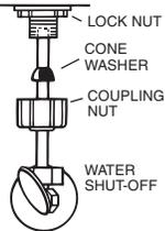
These parts must be used as illustrated to insure water-tight connection. Use of existing coupling nut may result in water leakage. Water supply tube or pipe must extend at least 1/2" inside threaded shank of valve (does not apply to flanged tubing).
