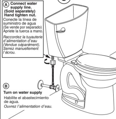
**WARNING: Overtightening of water supply line nuts could result in breakage and potential flooding.**
