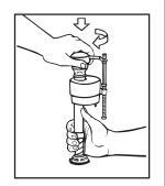
Replace TOP by engaging lugs and rotating 1/8 turn clockwise. MAKE CERTAIN TIP IS TURNED TO THE LOCKED POSITION. VALVE MAY NOT TURN ON IF TOP IS NOT FULLY TURNED TO THE LOCKED POSITION. **TROUBLESHOOTING**
