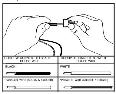
\*Note: When parallel wire is used, the tracer wire is square shaped or ridged and less tracer wire is round in shape or smooth. (Seen best when viewed from wire end.) To separate wires, grasp the ends of each wire and pull apart.
