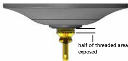
Drawing 2 Canopy Adjustment
