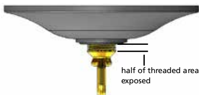
Drawing 2 Canopy Adjustment
