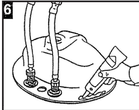
Squeeze a bead of sealant 1/4" from edge.
