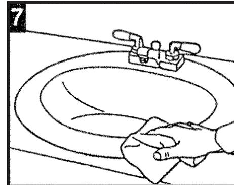
Set in position. Remove excess sealant with a damp rag.
